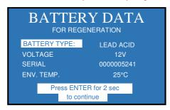
When all the fields are filled with valid values, keep pressed for at least two seconds to go to the OPERATING DATA display.
