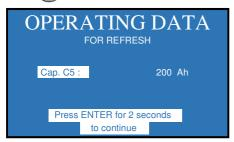
From anywhere on the BATTERY DATA and OPERATING DATA screens, press press for 2 seconds to go back to the MAIN MENU screen. The previous entered data will be lost.
