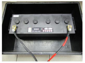
The use of pliers, clamps or other types of temporary connections is prohibited. Uncertain contacts could give rise to sparks in able to detonate the hydrogen produced by the battery under test.
