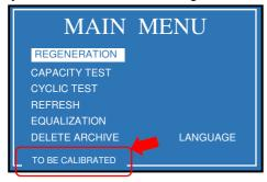
During operation, in the event of a fault or HW anomalies inside the system, the cycle in progress is interrupted and the display may have one of the following two screens, depending on the error found:
