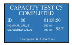
Near to the MEASURED VALUE there is the percentage of capacity reached at the end of the test with respect to the nominal one.
